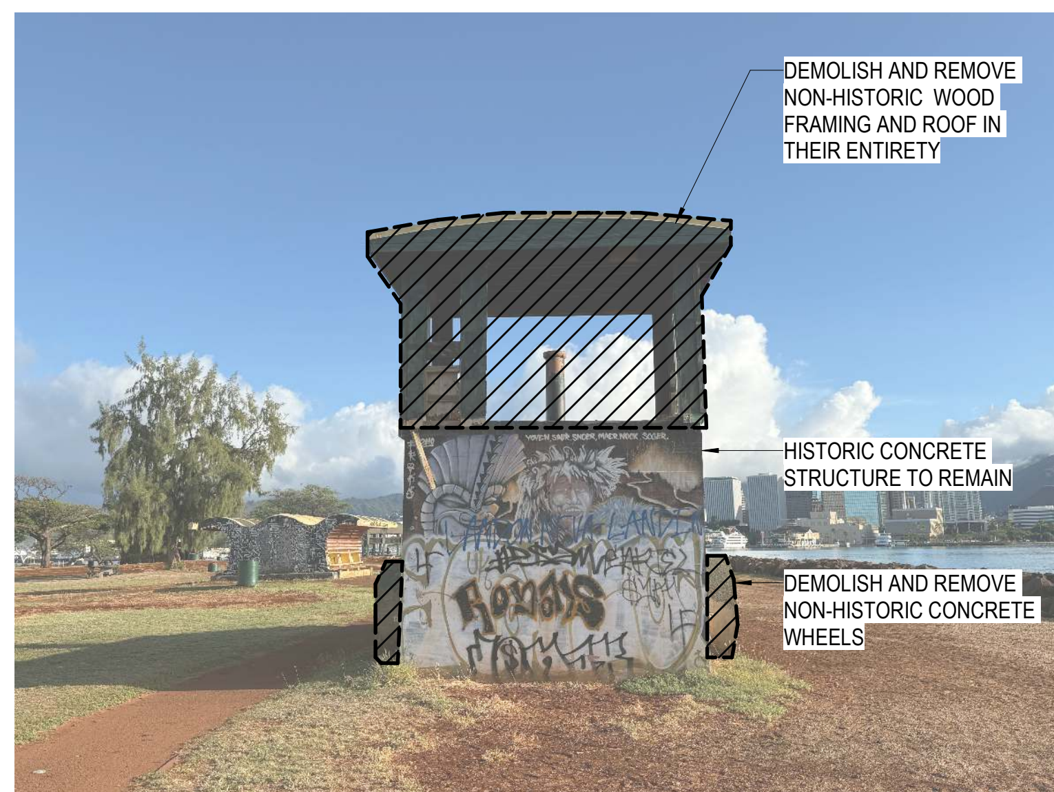
3 CABLE HUT (TRAIN)_SOUTH ELEVATION (PHOTO) SCALE: 3" = 1'-0"
